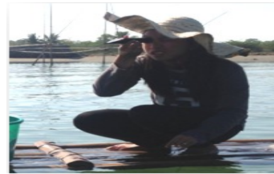
Measure water salinity using refractometer (left) and the temperature using thermometer (right).
