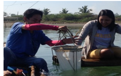
Measure plankton density using plankton net
