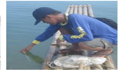
Measure water salinity using refractometer (left) and the temperature using thermometer (right).
